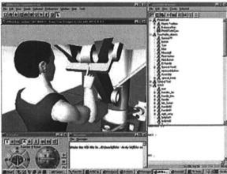
FIG. 7.7 Virtual prototyping environment showing the virtual world with the user's presence therein. Image courtesy of VP Group.
